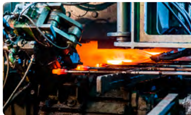
Die forming of sucker-rod heads at the ETCHHELLS line
