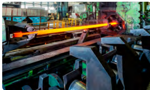
Pipe workpiece forging in the radial forging machine SXP-55 (GFM)
