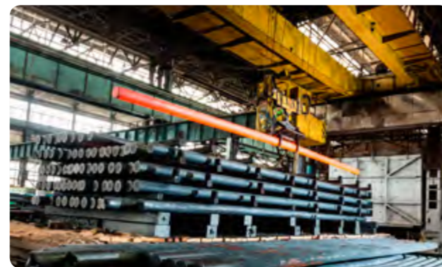
Pipe workpieces after heat treatment in the furnaces
