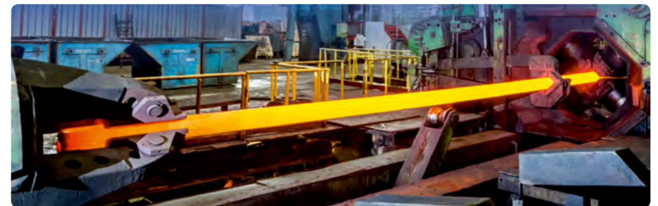
Pipe workpiece forging in the radial forging machine SXP-55 (GFM)
